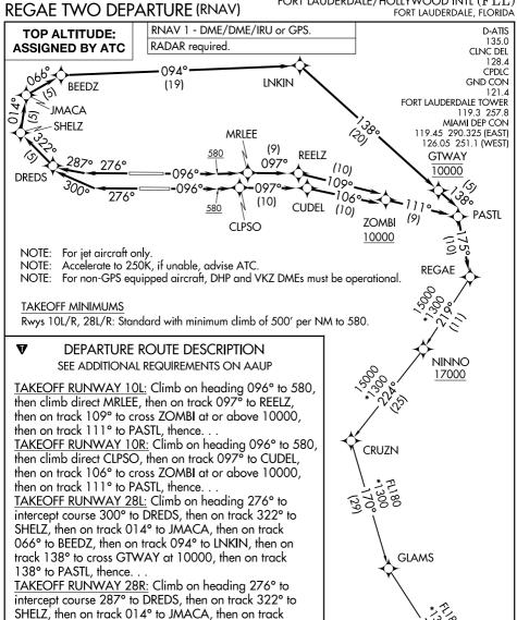
. . . on track 175° to REGAE, then on URSUS Transition. Maintain ATC assigned altitude. Expect clearance to filed altitude ten minutes after departure.
