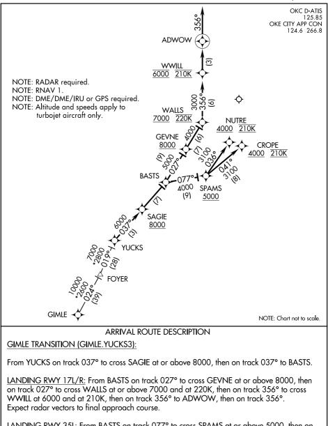
LANDING RWY 35L: From BASTS on track 077° to cross SPAMS at or above 5000, then on track 036° to cross NUTRE at or above 4000 and at 210K. Expect RNAV (RNP) approach.
