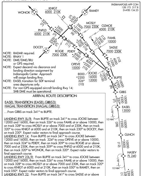
7000 and at 230K, then on track 321° to cross OZMOE at or above 4500 and at 210K. Expect RNAV (RNP), RNAV (GPS), or ILS or LOC RWY 32 approach
