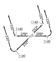
TAKEOFF MINIMUMS: Rwys 5, 10, 23, 28: Standard with minimum climb of 500' per NM to 1140.
